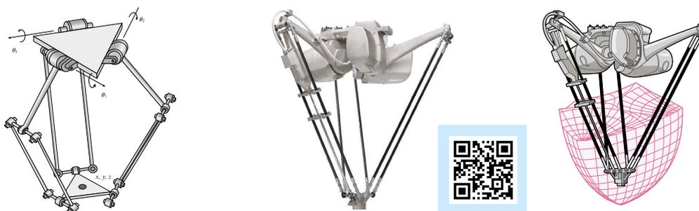
**Figure 5** Delta robot (Adapted from Benefeld et al., 2023: 27)
